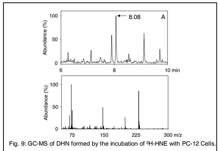
Fig. 9: GC-MS of DHN formed by the incubation of  $^3\text{H}$ -HNE with PC-12 Cells.
